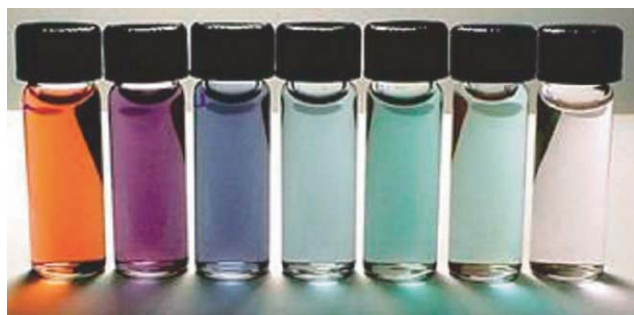
Fig. 10 Silica-cored gold nanoshell particles of various core-shell thicknesses demonstrating the variety of absorption wavelengths available through fine-tuning the particle geometry. (Reproduced with permission from: "Nanoshell-Enabled Photonics-Based Imaging and Therapy of Cancer," Technology in Cancer Research and Treatment , 2004, 3, 34. 26 Copyright 2004 Adenine Press, http://www.tcr.org/ )
